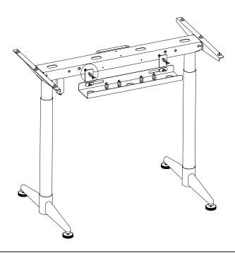
Step 1: Locate two screw holes on the backside of the beam and mount metal connector as illustrated below with two wing screws and washers, attach the tray to the metal connector with wing screws and slip adapters.
